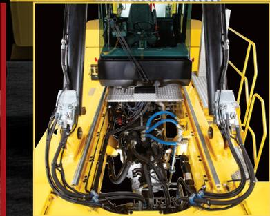
**THE EASILY REMOVABLE TOP DECK PLATES WITH QUICK DISCONNECT LATCHES PROVIDES FAST ACCESS TO MAJOR COMPONENTS.**
